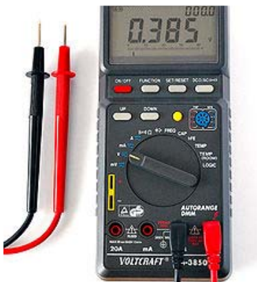
Multi-meter. A most useful tool for checking if circuits are hot when troubleshooting electrical equipment.
