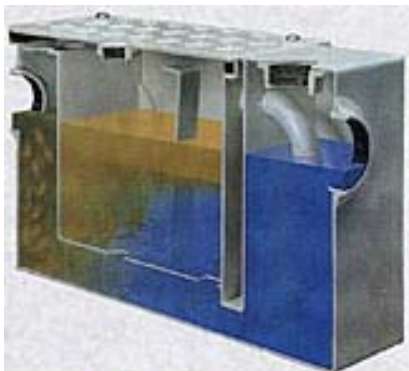
Typical under the sink style grease trap. Generally range in size from 80 to 150 liters per minute. Must be cleaned daily to prevent odor and clogging.
